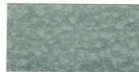
Galvanized G-90 SRI-65 Metallic coating over steel. No finish warranty, no perforation warranty
